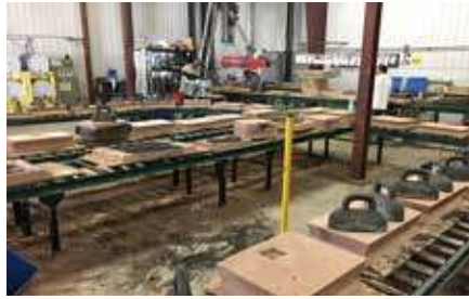
NO BAKE / "AIRSET" FOUNDRY OPERATIONS
